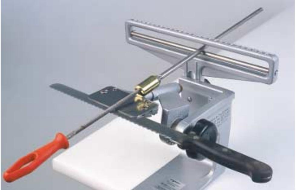
Photo shows round file to suit the serration of serrated edge knife to be sharpened. Different files are used for different serration sizes.
